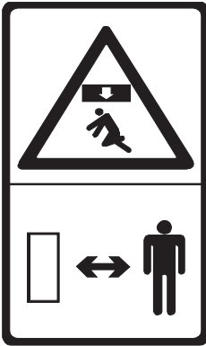
15 WARNING! Raised attachment, keep a safe distance from the machine.
