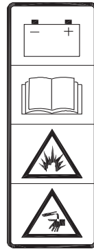
14 WARNING! Risk of electrical shock, corrosive burns and explosion – read the Operator's manual.
